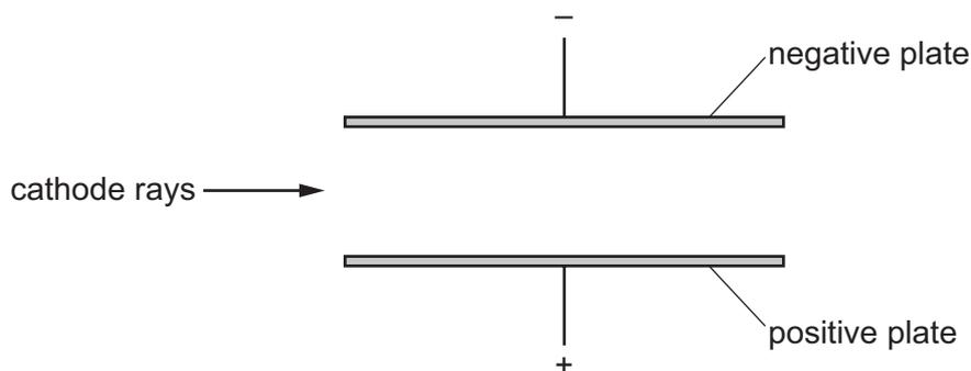
The cathode rays are deflected as they pass between the plates.
