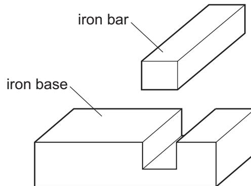
At room temperature, the bar is slightly too big to fit in the gap.
